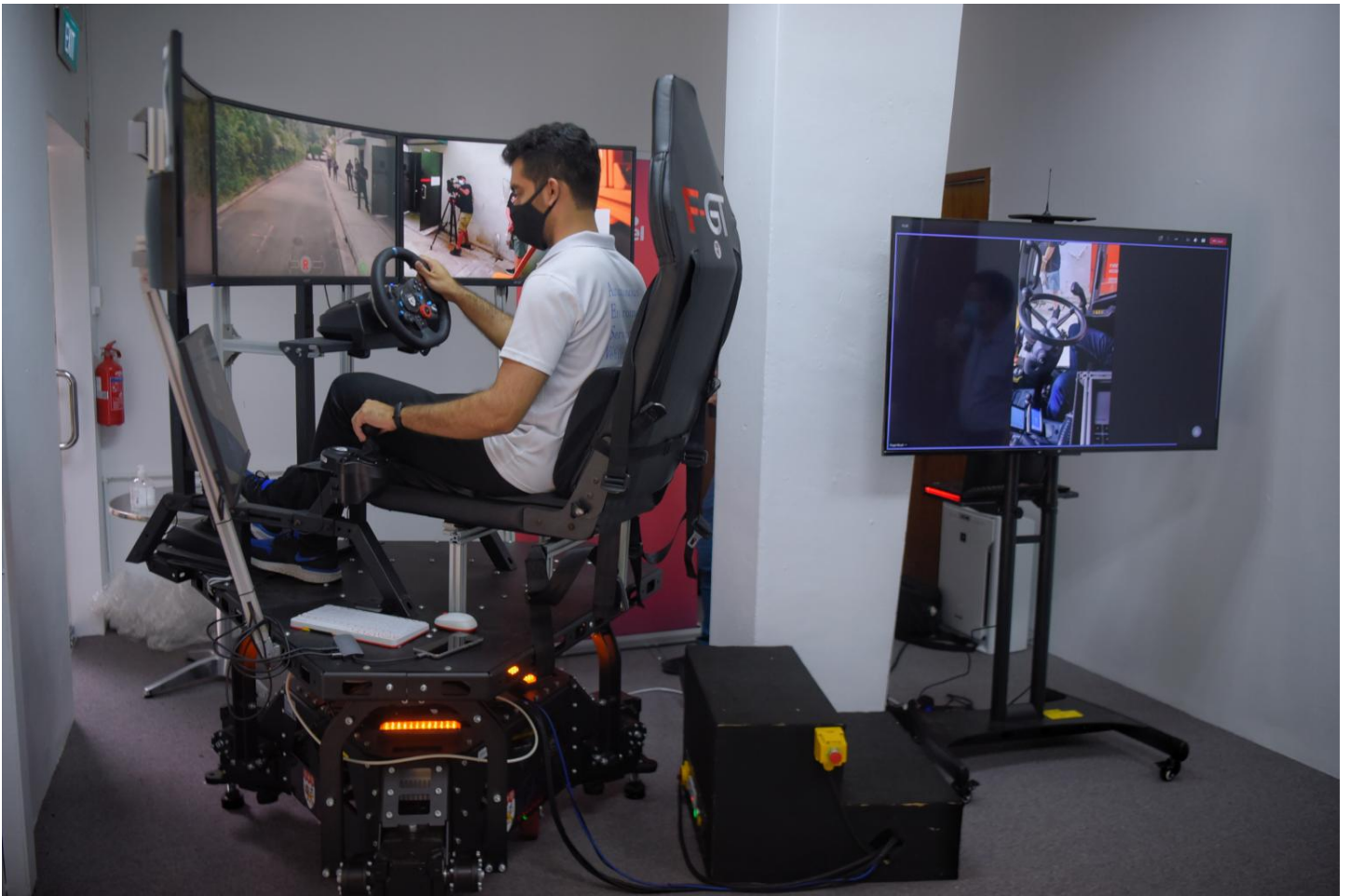
The teleoperation system that an operator uses to control the roadsweeper looks akin to a driving simulator and creates the illusion that he is sitting in the actual vehicle in Sentosa. ST PHOTO: MARK CHEONG
