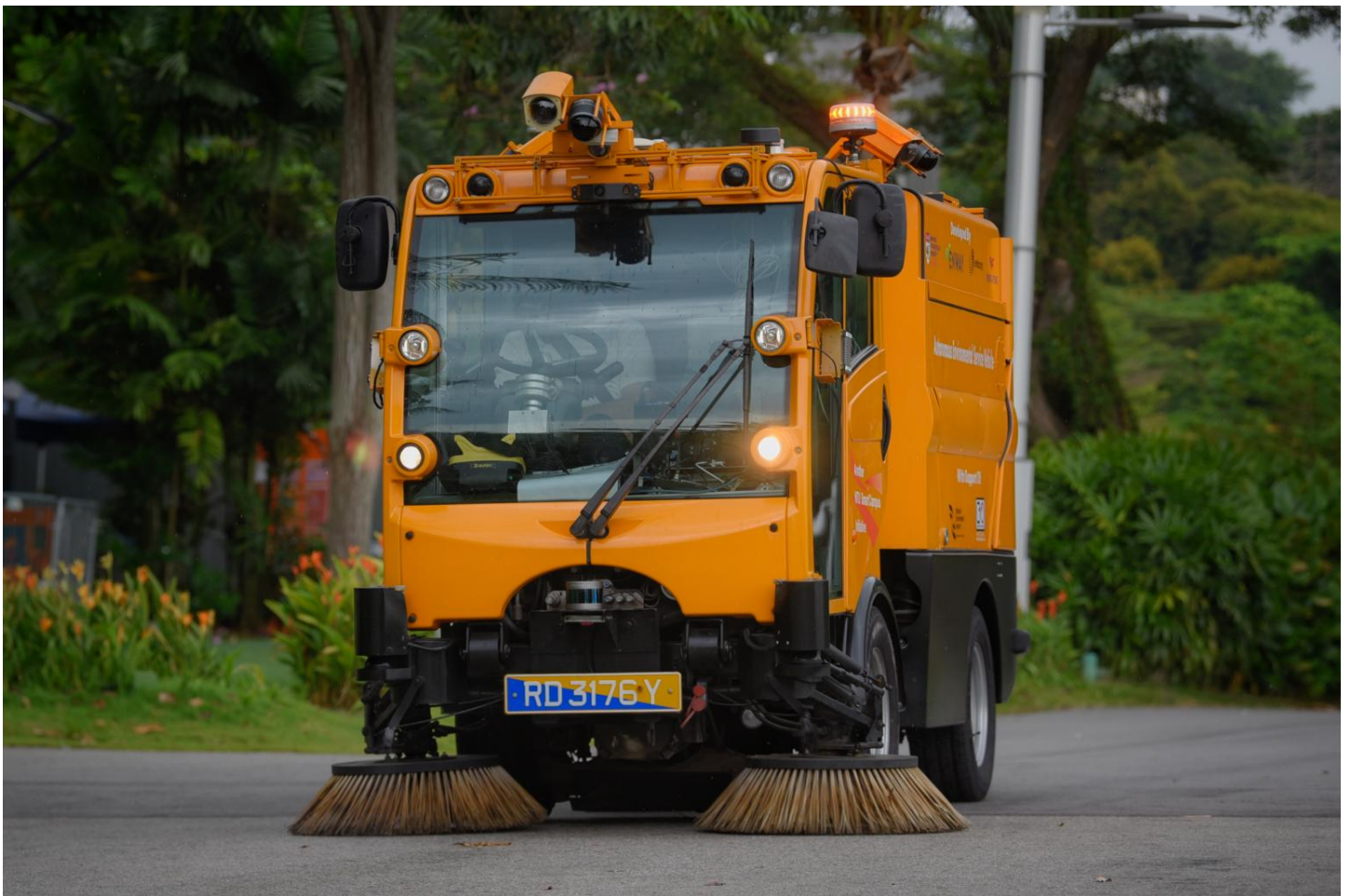
A driverless roadsweeper vehicle in Sentosa. The vehicle can be controlled by an operator from elsewhere. ST PHOTO: MARK CHEONG
